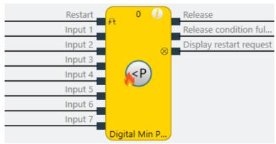
Illustration 204: Logical connections for the Digital min pressure function block
