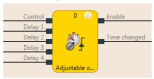
Illustration 88: Function block diagram for the adjustable switch-on delay function block
