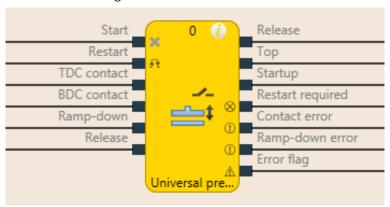
Illustration 138: Logical connections for the universal press contact monitor function block
