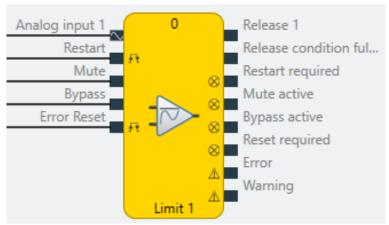
Illustration 169: Logical connections for the limit function block
