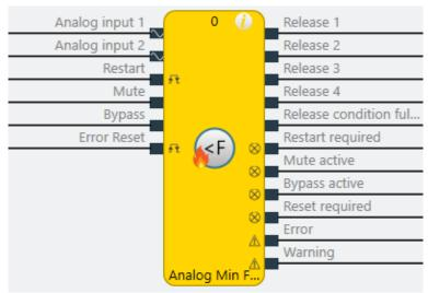
Illustration 187: Logical connections for the Analog min flow function block
