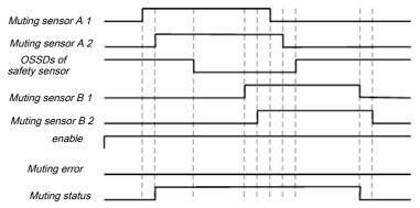
Illustration 122: Valid muting sequence when using the basic configuration setting
