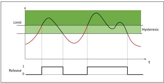
Illustration 198: Monitoring for "Lower limit exceeded"
