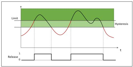
Illustration 183: Monitoring for "Lower limit exceeded"
