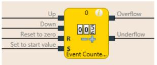
Illustration 58: Logical connections for the counter function block (up and down)
