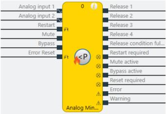
Illustration 181: Logical connections for Analog min pressure function block
