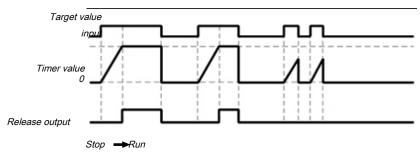
Illustration 87: Sequence/timing diagram for the switch-on delay function block
