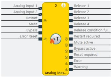
Illustration 196: Logical connections for the Analog max temperature function block
