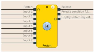
Illustration 80: Function block diagram for the restart function block
