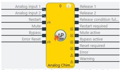
Illustration 199: Logical connections for analog chimney draught function block
