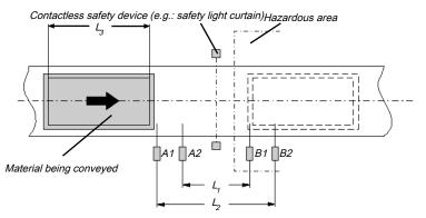
Illustration 124: Example of the sequential arrangement of muting sensors
