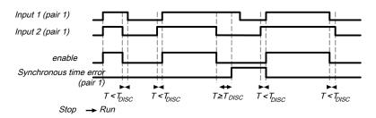
${\it Illustration 111: Sequence/timing\ diagram\ for\ switch\ evaluation\ function\ block,\ category\ 4,\ two-channel\ without\ function\ test}$
