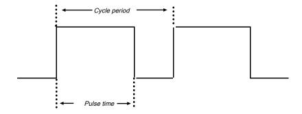
Illustration 56: Parameter diagram for the "Cycle generator" function block
