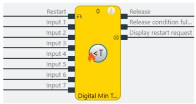
Illustration 212: Logical connections for the Digital min temperature function block
