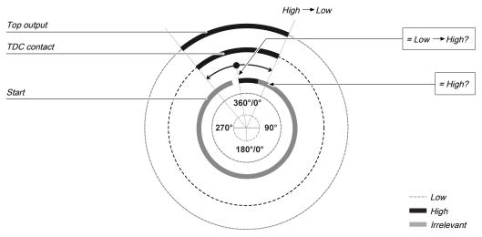
Illustration 134: Ramp-down monitoring with the eccentric press contact monitor function block
