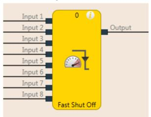
Illustration 59: Logical connections for the fast shut-off function block
