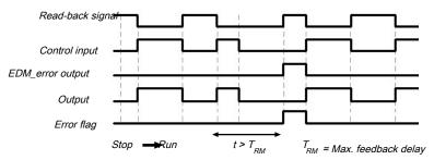
Illustration 91: Sequence/timing diagram for the EDM function block
