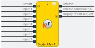
Illustration 210: Logical connections for the Digital max flow function block
