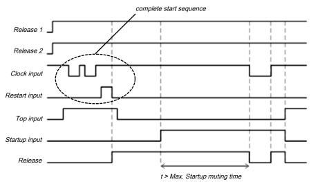
Illustration 164: Sequence/timing diagram if the Cycle input is low, maximum startup muting time > 0, and restart interlock set to 3 - After shutdown in downstroke or initial position.
