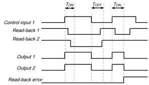
Illustration 94: Sequence/timing diagram for double valve in manual reset mode
