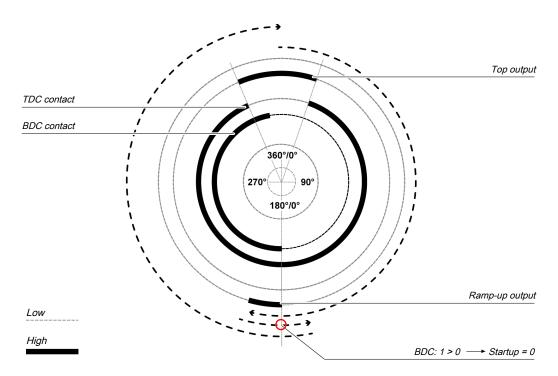
Illustration 143: Press cycle for the universal press contact monitor function block with 2 BDC transitions
