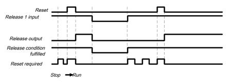
Illustration 213: Flow/Timing diagram for the function block
