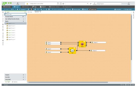
Illustration 31: Adding inputs and outputs to a grouped function block
