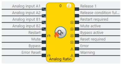
Illustration 203: Logical connections for the Analog Ratio function block
