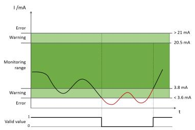
Illustration 40: Example: Value below lower limit of monitoring range (sensor 4-20mA)
