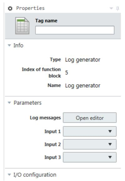
Illustration 76: Assignment of the input conditions for the log generator function block
