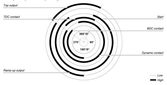
Illustration 137: Contact and output sequence of an eccentric press during an error-free sequence (example)
