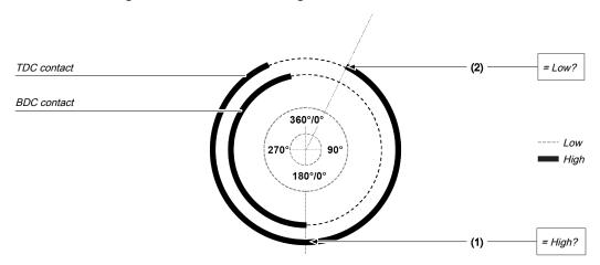
Illustration 140: Contact monitoring with the universal press contact monitor function block with activated BDC contact
