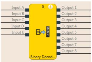
Illustration 70: Logical connections for the binary decoder function block
