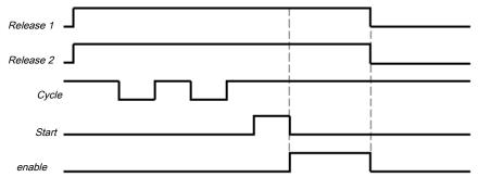
${\it Illustration 159: Cycle/timing\ diagram\ for\ a\ complete\ start\ sequence\ in\ standard\ mode\ in\ two-cycle\ operation}$
