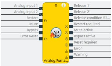
Illustration 201: Logical connections for the analog furnace pressure function block
