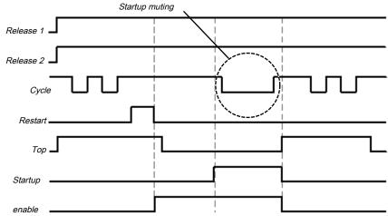
Illustration 161: Sequence/timing diagram for startup muting in standard mode in two-cycle mode
