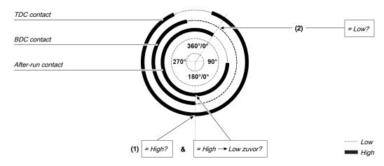
${\it Illustration 145: Contact\ monitoring\ with\ the\ universal\ press\ contact\ monitor\ function\ block\ with\ activated\ BDC\ contact\ and\ ramp-down}$
