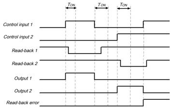
Illustration 95: Sequence/timing diagram for directional valve
