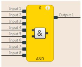
Illustration 49: Function block diagram for the AND function block
