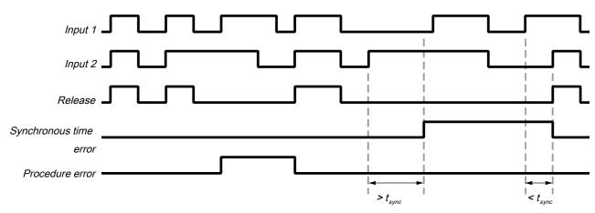
Illustration 106: Sequence/timing diagram for the emergency stop function block
