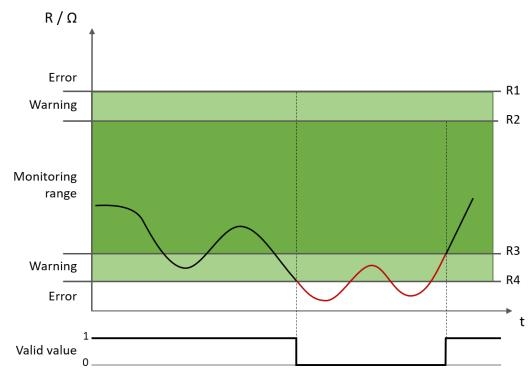
Illustration 42: Example: Value below lower limit of monitoring range (sensor RTD)
