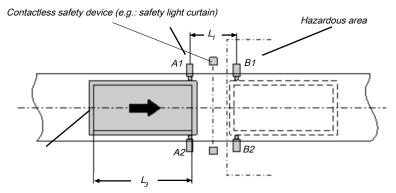
Illustration 121: Muting with two parallel sensor pairs
