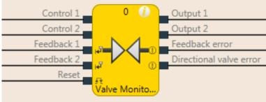
Illustration 92: Logical connections for the valve monitoring function block configured for a directional valve
