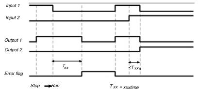
Illustration 97: Sequence/timing diagram for the mode selection switch function block
