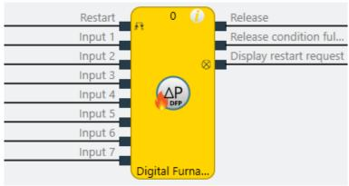
Illustration 218: Logical connections for the digital furnace pressure function block
