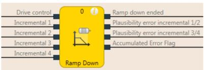
Illustration 98: Logical connections for the ramp down detection function block
