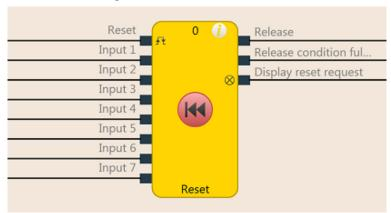
Illustration 78: Function block diagram for the reset function block
