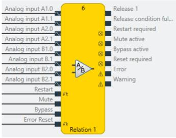
Illustration 174: Logical connections for the ratio function block
