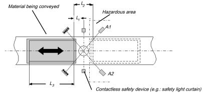
Illustration 130: Cross muting (two sides) with bidirectional movement of material
