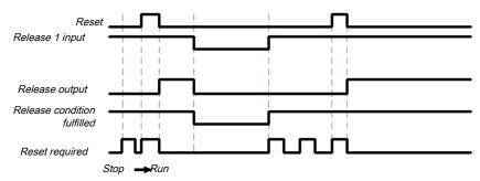
Illustration 81: Sequence/timing diagram for the restart function block
