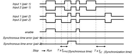
Illustration 114: Sequence/timing diagram for the two-hand type IIIC function block
