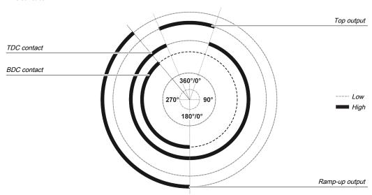
Illustration 142: Press cycle for the universal press contact monitor function block with falling edge of BDC contact before TDC contact
