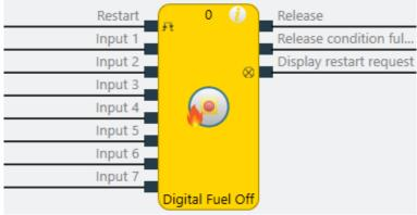
Illustration 220: Logical connections for the Digital fuel off function block
