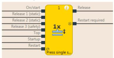
Illustration 150: Logical connections for the press single stroke function block
