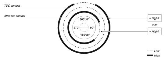
Illustration 139: Contact monitoring with the universal press contact monitor function block with activated ramp-down
