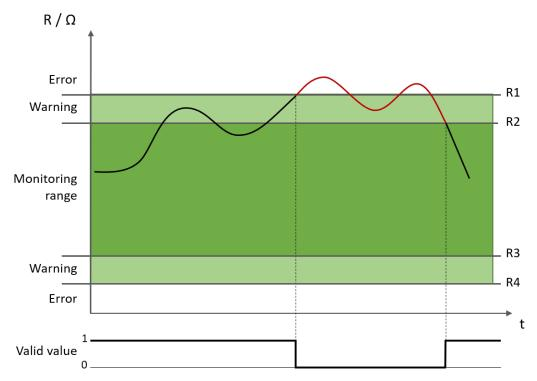
Illustration 43: Example: Value above upper limit of monitoring range (sensor RTD)
