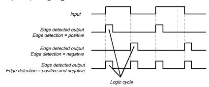
Illustration 68: Timing diagram for the edge detection function block
