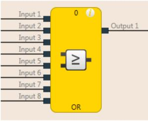
Illustration 50: Function block diagram for the OR function block
