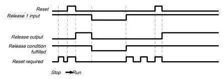
Illustration 205: Flow/Timing diagram for the function block
