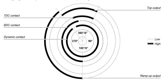
Illustration 135: Press cycle for the eccentric press contact monitor function block with dynamic contact on the upstroke
