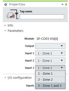
Illustration 63: Parameter settings for the fast shut-off function block
