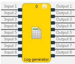
Illustration 72: Function block diagram for the log generator function block
