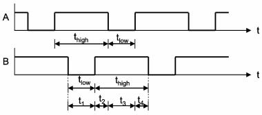
Illustration 100: Signal pattern for 1/3 gap pulse encoder with 180° phase offset
