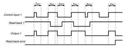
Illustration 93: Sequence/timing diagram for single valve in manual reset mode
