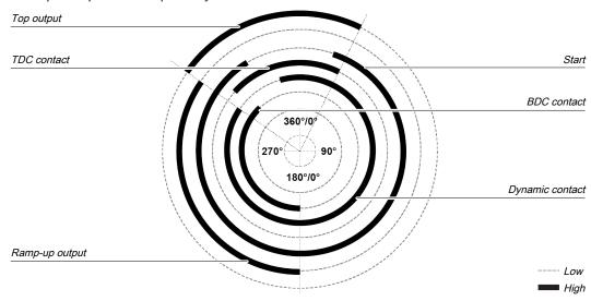
Illustration 146: Contact and output sequence of a universal press during an error-free sequence (example)
