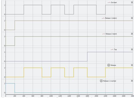
Illustration 148: Typical sequence/timing diagram for the press setup function block
