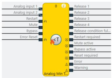
Illustration 193: Logical connections for the Analog min temperature function block
