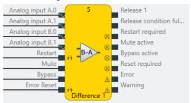
Illustration 175: Logical connections for the difference function block
