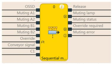
Illustration 123: Logical connections for the range function block Sequential muting
