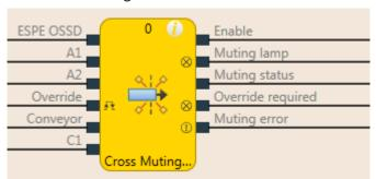
Illustration 126: Logical connections for the Cross muting (one side) function block with the C1 input
