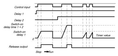
Illustration 89: Sequence/timing diagram for the adjustable switch-on delay function block with switch-on delay time 1 and switch-on delay time 2
