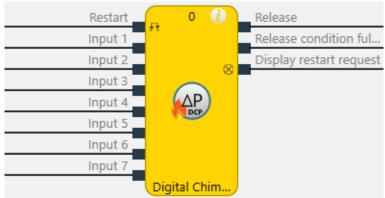
Illustration 216: Logical connections for the Digital chimney draught function block
