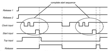
${\it Illustration 163: Sequence/timing\ diagram\ if\ the\ Cycle\ input\ is\ low,\ startup\ muting\ inactive,\ and\ restart\ interlock\ set\ to\ {\it 2-always}.}$
