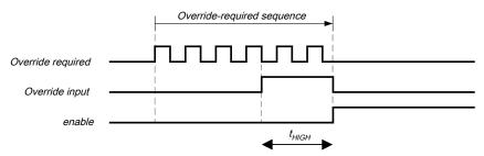
Illustration 119: Logic diagram for override and override requirement
