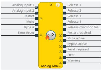
Illustration 184: Logical connections for the Analog max pressure function block
