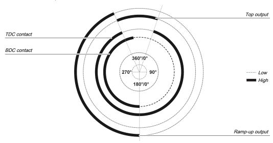
Illustration 141: Press cycle for the universal press contact monitor function block with falling edge of **TDC contact** before **BDC contact**
