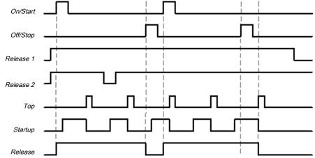
Illustration 156: Typical sequence/timing diagram for the press automatic function block
