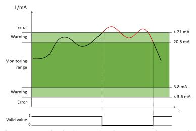
Illustration 41: Example: Value above upper limit of monitoring range (sensor 4-20mA)
