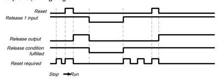
Illustration 79: Sequence/timing diagram for the reset function block
