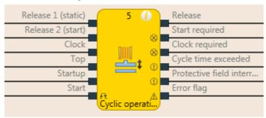
Illustration 157: Logical connections for the cyclic operation function block
