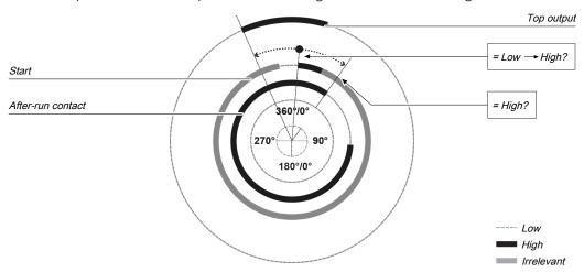
Illustration 144: Ramp-down monitoring with the universal press contact monitor function block
