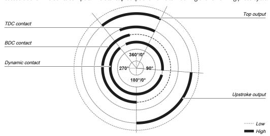
Illustration 136: Press cycle for the eccentric press contact monitor function block with dynamic contact at startup and for the downward movement
