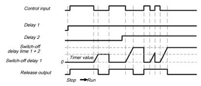
Illustration 85: Sequence/timing diagram for the adjustable switch-off delay function block with switch-off delay time 1 and switch-off delay time 2
