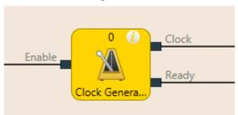
Illustration 55: Logical connections for the cycle generator function block
