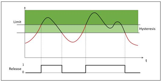
Illustration 192: Monitoring for "Lower limit exceeded"
