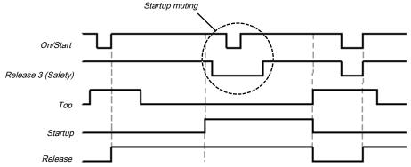
Illustration 152: Sequence/timing diagram for the press single stroke function block startup muting of On/Start and Release 3 (safety)
