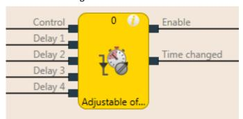
Illustration 84: Function block diagram for the adjustable switch-off delay function block
