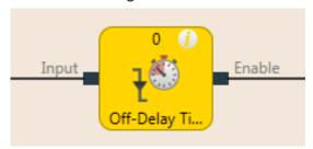
Illustration 82: Function block diagram for the switch-off delay function block
