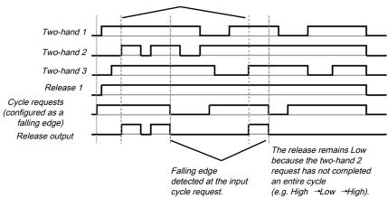
Illustration 116: Sequence/timing diagram for the multi-two-hand function block
